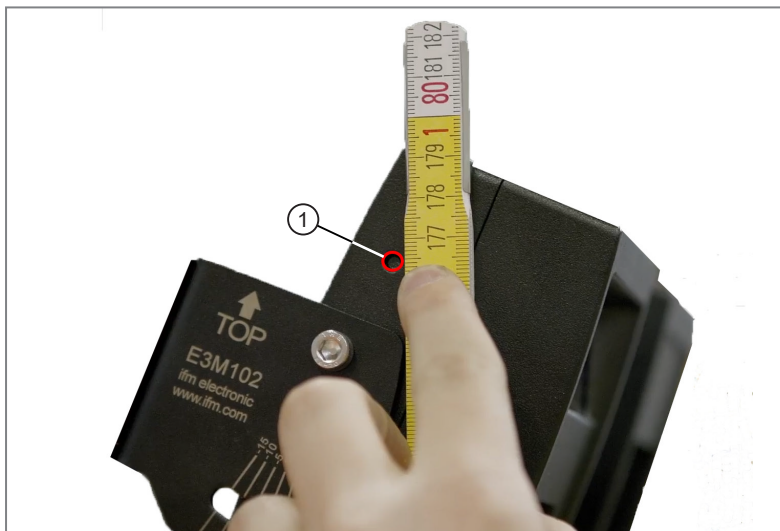
Fig. 29: Measuring the inclination angle via the reference socket
