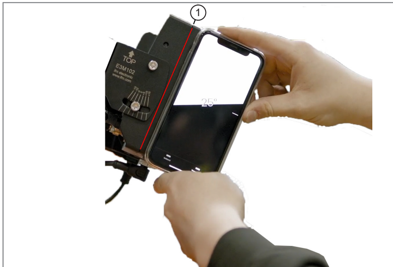
Fig. 28: Measuring the inclination angle with a smartphone
